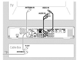
The cable box have to be connected **before** the DVD-Recorder (cable box - DVD-Recorder - TV set). On the jack **TV OUT** only the TV have to be connected.
